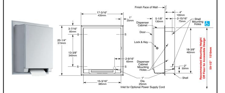
Rough Wall Opening 16" (405mm) wide 18-7/8" (480mm) high 4" (102mm) minimum recessed depth
