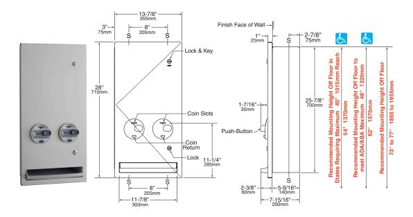
Rough Wall Opening 12-1/2" (320mm) wide 26-3/8" (670mm) high 5-9/16" (140mm) minimum recessed depth
