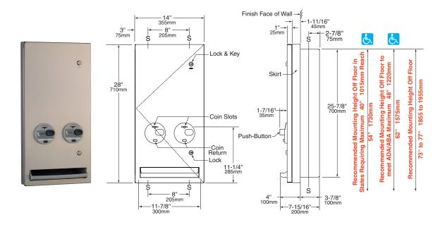
Rough Wall Opening 12-1/2" (320mm) wide 26-3/8" (670mm) high 3-7/8" (100mm) minimum recessed depth
