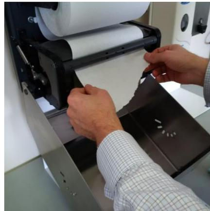
Step 5: Crease paper along the top of the internal roller with rubber face
