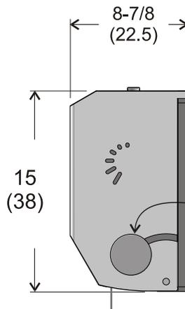
Paper advance wheel for loading paper and alternate feeding of paper.
