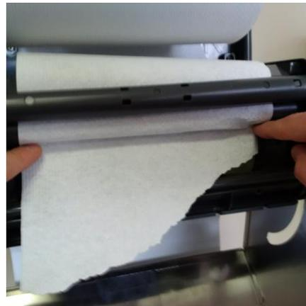
Step 6: Provide some pressure against the crease of paper and turn the knob on the outside of the unit clockwise
